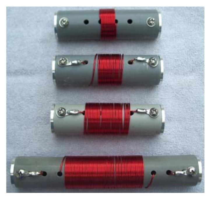
Pictured above are the loading coils for 17m, 20m, 30m, and 40m (top to bottom). As stated above, the basic kit comes with parts and wire to assemble two coils, one on the 3.5" coil, and one on the 6" coil. You can choose any two bands between 10m and 60m. Detailed instructions are given for each band on the number of needed turns and the correct manner to wind them.
