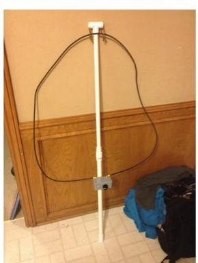
The final step is to attach all the connectors. I attached the smaller conductor to a BNC binding post connector. I attached the terminal connectors to the Coax and I was in business. Place the binding post over the brass bolt, put it through the loop guides and attach on the other end. I attached the smaller loop in the plane of the outer loop and attached it to the top of the form. I fired up the radio and. . .
